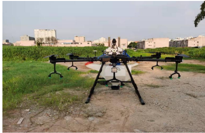
FIGURE 0-1 HYBRID LARGE CAPACITY SPRAY DRONE
